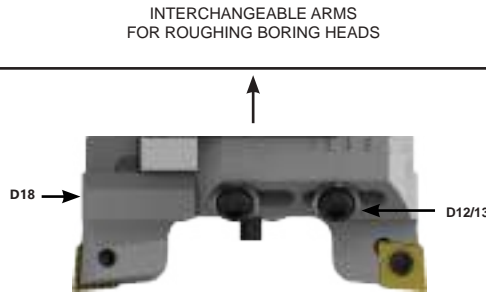
INSERT NO. 1 FIRST CUT SMALLER AND DEEPER CUT INSERT NO. 2 SECOND CUT LARGER AND SHALLOW CUT
